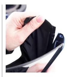
**6.3** Unfasten the face seal by pulling its frame until the pins release from the holes in the visor.
