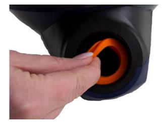
**8.2** Remove the gasket from the flange.
